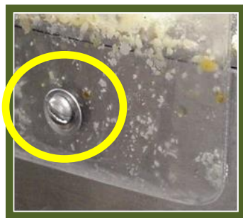
Figure 15. Splashguard requiring tool for disassembly and creating a catch point
