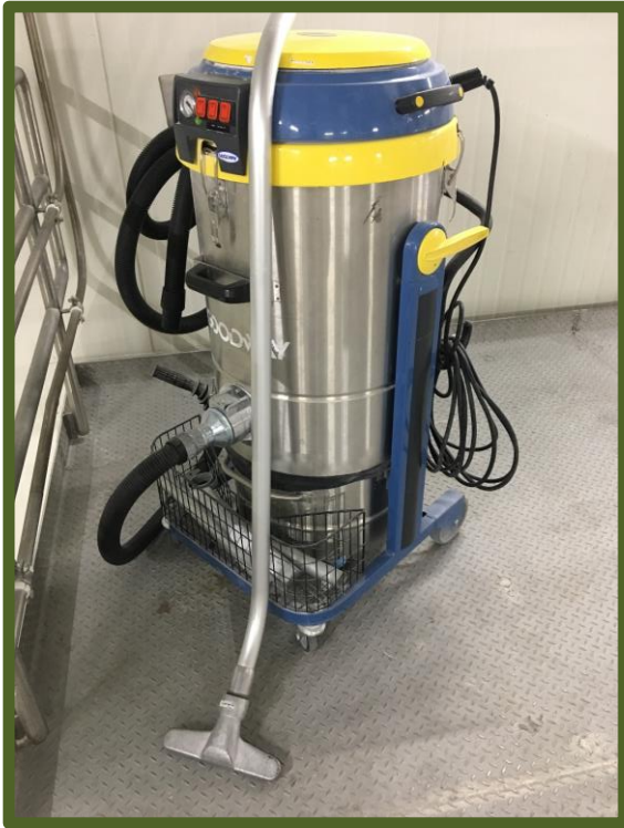
Figure 30. Dedicated HEPA filtered vacuum cleaners.
