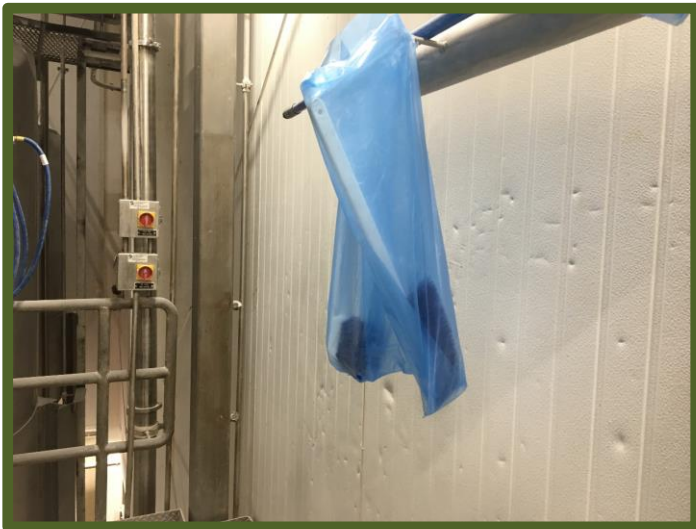
Figure 32. Product contact brushes stored in blue bags after cleaning until next use
