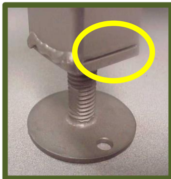
Figure 21. Hollow square tubing not hermetically
