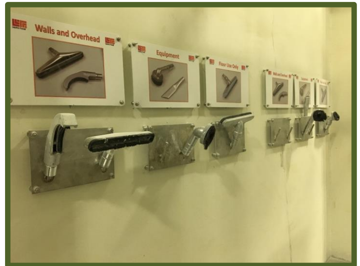
Figure 33. Vacuum attachments designated by shape rather than by color
