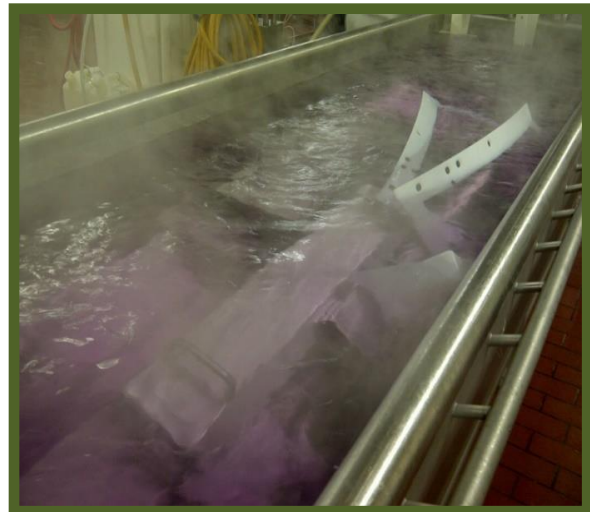
Figure 28. Equipment must be fully submerged for appropriate cleaning.
