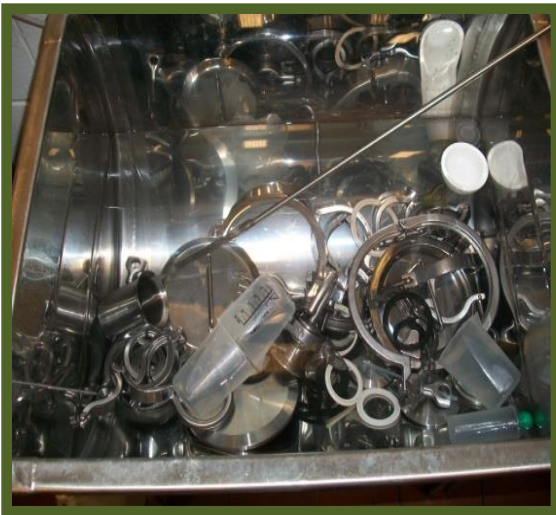
Figure 27. Incorrect storage of parts in a COP tank. They should be stored in designated receptacles and/or areas.
