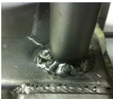
Fig. 11. Poor sanitary welds are not cleanable at a microbiological level
