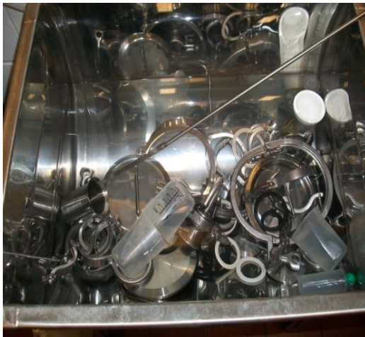
Fig. 27 Incorrect storage of parts in a COP tank. They should be stored in designated receptacles and/or areas
