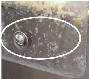
Fig 15. Splashguard requiring tool for disassembly and creating a catch point
