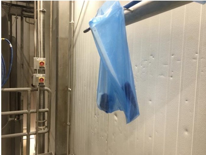
Fig. 32. Product contact brushes stored in blue bags after cleaning until next use.
