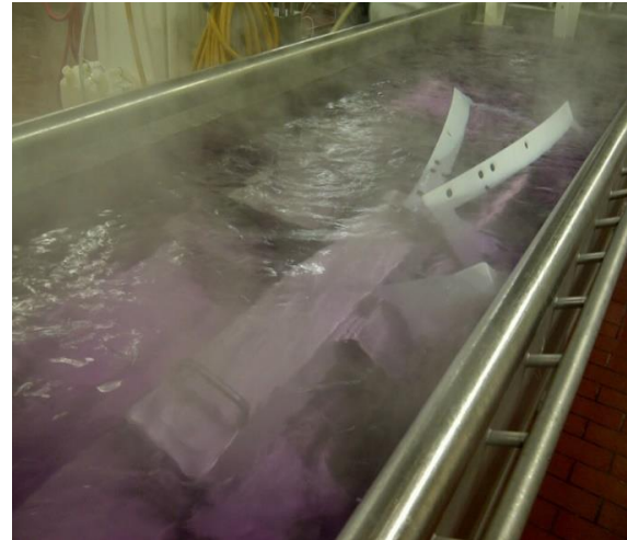
Fig.28. Equipment must be fully submerged for appropriate cleaning
