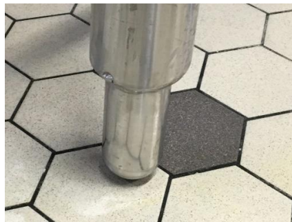
Fig. 22. Example of adjustable ball foot design – welded or gasket to seal and avoid debris infiltration
