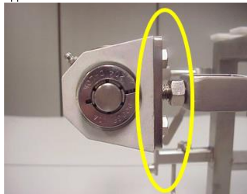
Fig. 37. Sandwich area formed by the bearing housing and framework where Listeria spp. had established a niche and the framework had rusted
