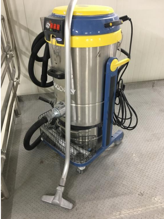
Fig. 30. Dedicated HEPA filtered vacuum cleaners.
