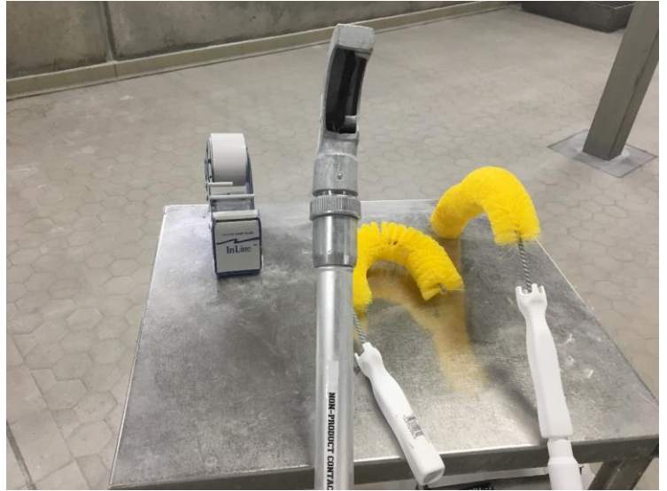
Fig. 31. Overhead pipe exterior cleaning tools.
