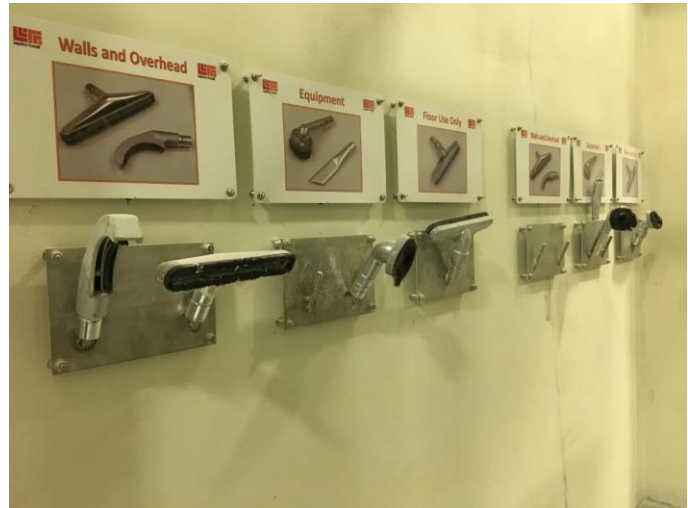
Fig. 33. Vacuum attachments designated by shape rather than by color.
