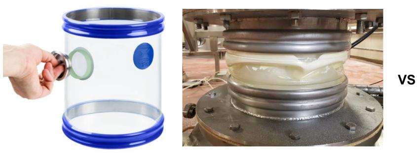
BFM connections with complete **seal vs. clamped** connections that develop niche or powder ingress / egress These can also be used for CIP return connections and sampling
