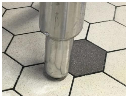
Fig. 21. Example of adjustable ball foot design – welded or gasket to seal and avoid debris infiltration
