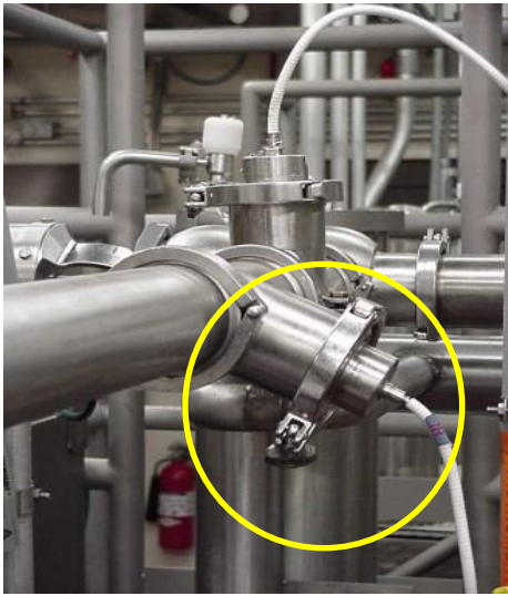
Fig. 22. Accumulation/niche created by reassembling the probe facing down instead of up
