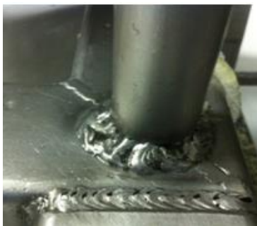
Fig. 10. Poor sanitary welds are not cleanable at a microbiological level
