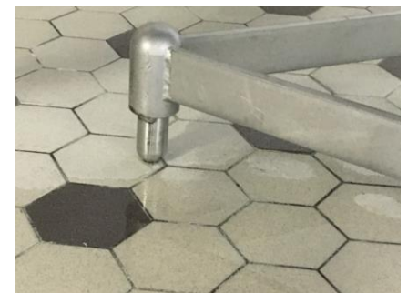
Fig. 21. Example of adjustable ball foot design – welded or gasket to seal and avoid debris infiltration
