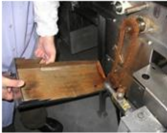
Fig. 12. Example of material incompatible with cleaning solution / method
