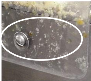
Fig 14. Splashguard requiring tool for disassembly and creating a catch point
