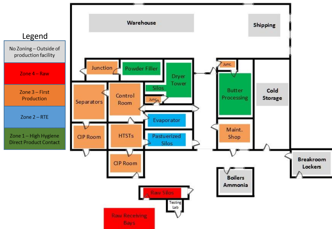
Fig. 3. An example of a Powder and Butter operation with hygiene zoning and hygiene junction rooms/airlocks
