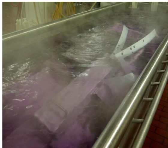
Fig.27. Equipment must be fully submerged for appropriate cleaning
