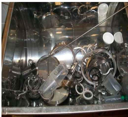
Fig. 26 Incorrect storage of parts in a COP tank. They should be stored in designated receptacles and/or areas
