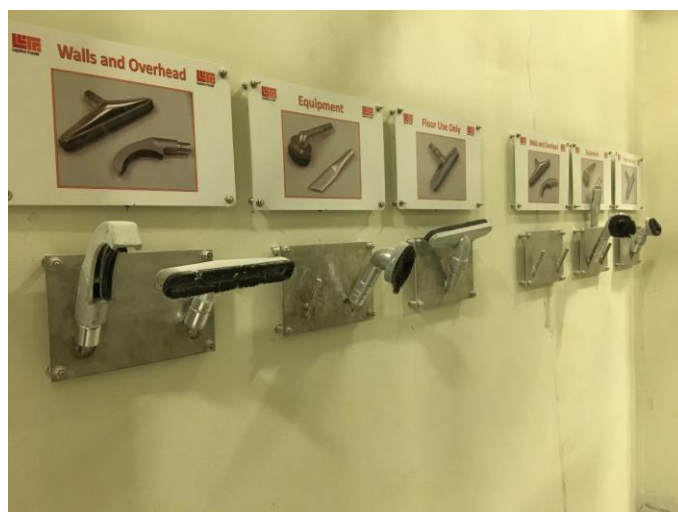
Fig. 32. Vacuum attachments designated by shape rather than by color.
